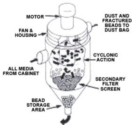
Reclaimer separates the glass beads. Returns only the round beads to the system. Exhausts dirt, broken beads, etc. to the dust bag.
